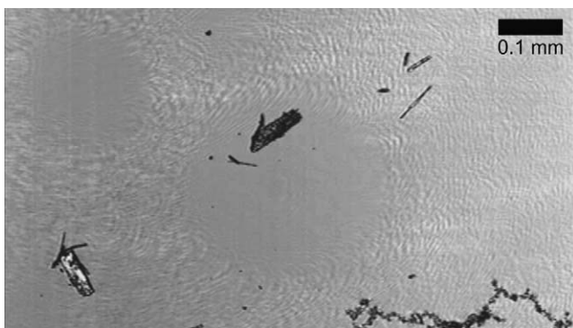
Fig. 6. Micrograph from the confocal microscope, showing the Wollastonite fibers on top of the glass at 800^\circ\text{C} . Note the debris at the bottom right, which does not nucleate crystals during the experiment.
